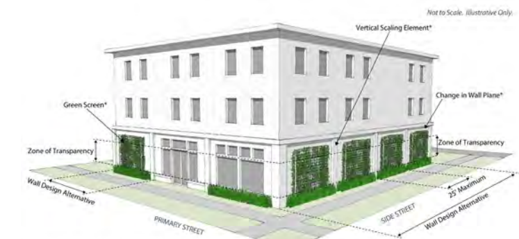
*Green Screen, Vertical Scaling Elements, and Change in Wall Plane create a system of wall design elements. Transparency Alternative: Wall Design Elements
